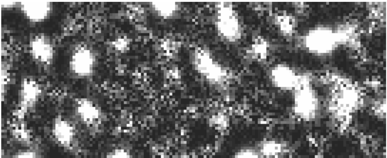
Figure 2: (a) (top panel): A subsection of the test image. The circles mark known positions of stars. (b) (centre panel): The same subsection after 20 iterations of Lucy-Richardson deconvolution. Several star-like artifacts appear near the centre. (c) (bottom panel): The same as (b), but with different noise pattern. The artifacts are at positions different from those in (b).
